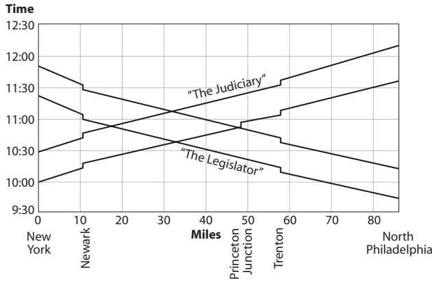
Figure 5.7 Four trains on the track: New York–Philadelphia.
